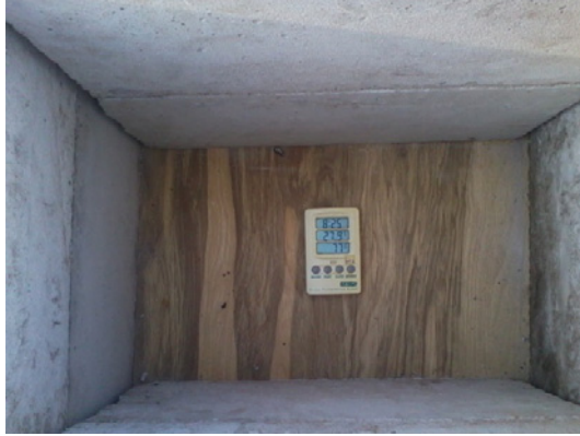
Figure 2. Temperature reading inside of concrete block model
