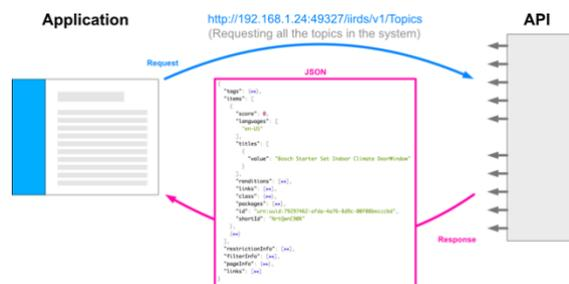
**Fig. 8.** Schematic representation of the transaction between the application and the iiRDS API.
