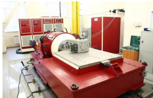
**Figure 4.** Vibration Test System DataPhysics, LE-2016/DSA10-200K
