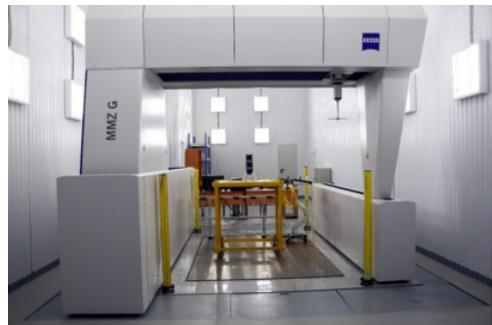
**Figure 6.** Coordinate Measuring Machine
