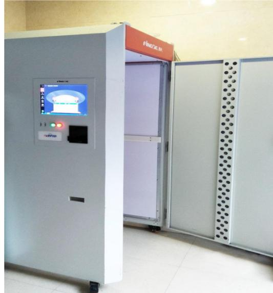
**Figure 4.** RFID scanning cabinet
