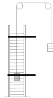
Figure 4. Two rubber bands are marked on the cylinder, and the cube passes through two rubber bands to record the time
