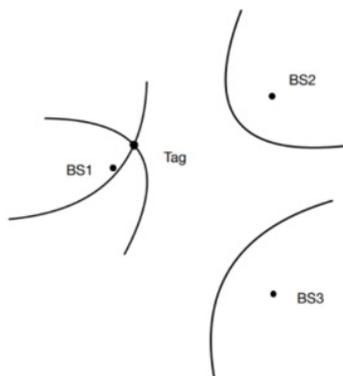
Figure 4 The positioning model of TDOA
