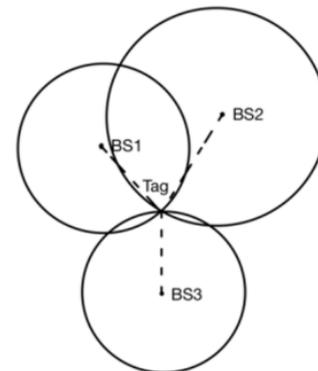
**Figure 3** The ideal positioning model of TOA in two-dimensional space
