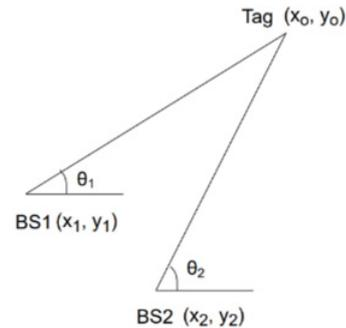
**Figure 2** The positioning model of AOA
