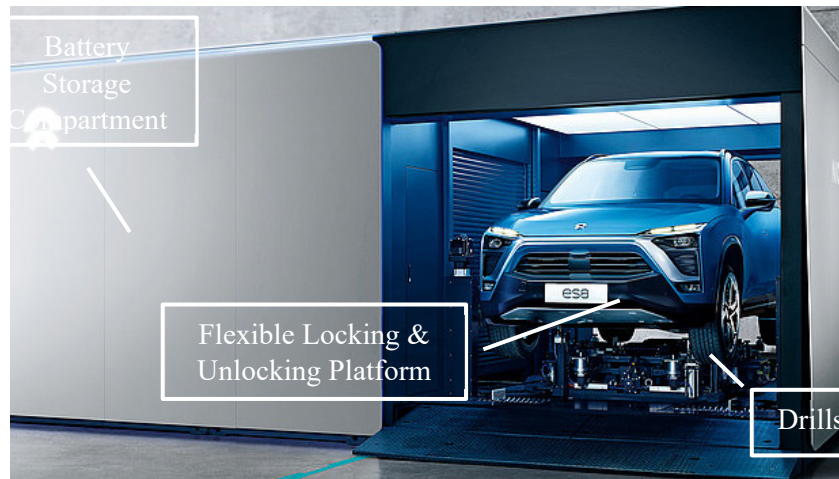
Figure 1 Labeled concept drawing of battery swap station developed by NIO [3]
