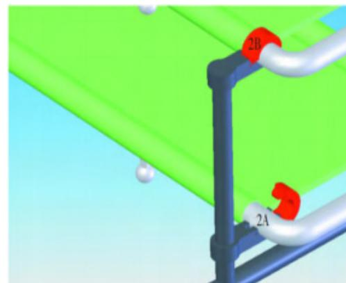
Note: 2A indicates open state and 2B indicates locked state
