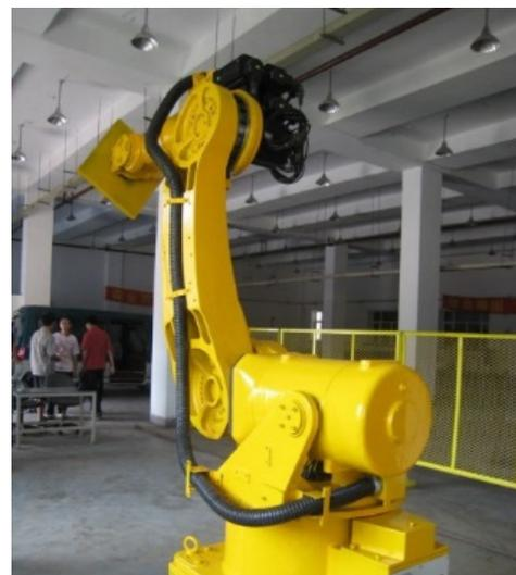
**Figure 4** QH-165 Spot Welding Robot
