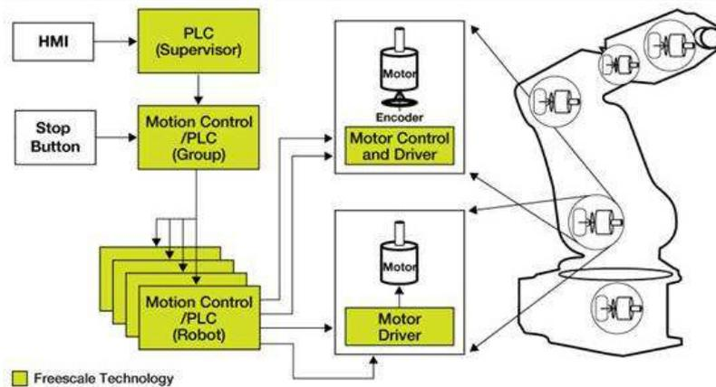
**Figure 1.** Industrial Robot Structure Block Diagram
