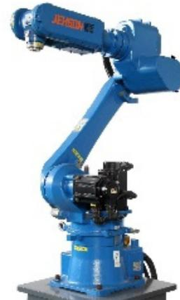
Figure 6 Six-axis articulated robot
