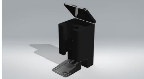
Figure 4. Charging Pod Design with Dust Container
