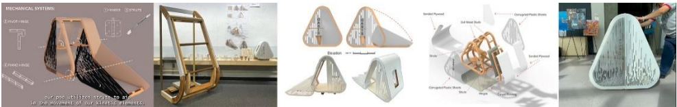
Fig. 8. Initial design proposal, segment of a full-scale construction to test hinge and tension spring system’s effectiveness and final 50% scale model.
